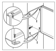
Remove the correct part from the 5. hinge cover (E). Make sure to remove the part DX, in the case of right hinge, SX in opposite case.
